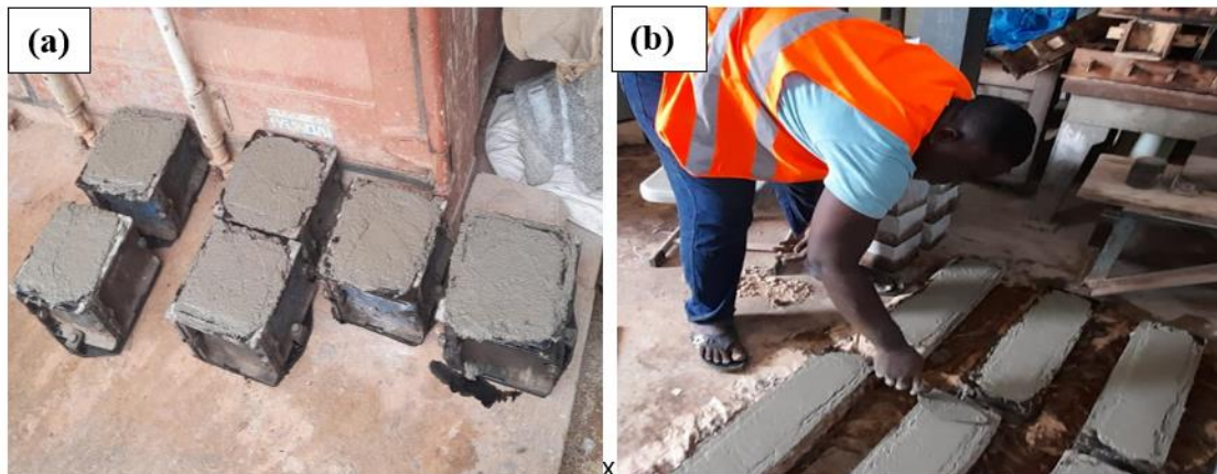
Fig. 2. Specimens: (a) concrete cubes, (b) concrete prisms
