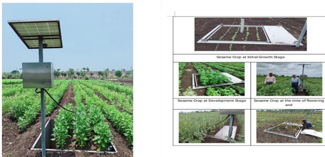
Fig. 2. Digital weighing lysimeter for estimation of Crop Evapotranspiration
